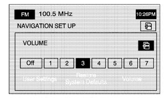
Restore System Defaults: Select this option from the NAVIGATION SET UP screen to change all adjustable system settings to factory defaults.
